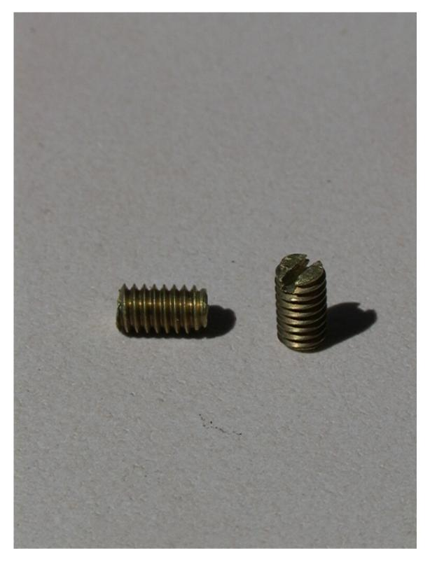
Note that the length of the grub screws was such that they would be recessed into the assembly when screwed home, like the one on the left in the photo below.
